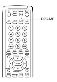
Press DRC-MF repeatedly DRC-MF until you receive the desired picture quality.
